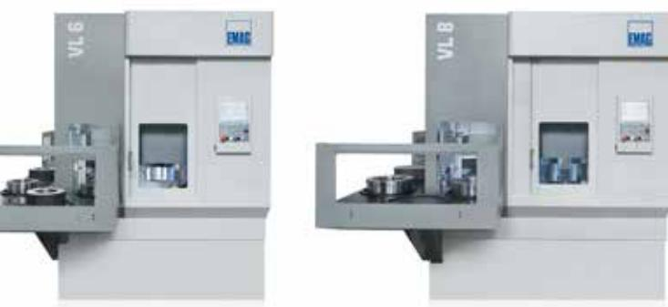
The smallest machine is the VL 2, designed for chucked parts up to 100 mm in diameter. It is followed by the machines VL 4, VL 6, and VL 8. The size of the workpieces they can handle increases by 100 mm with each model (up to 400 mm).
